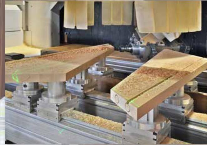
5-axes unit with cardanic 24 kW spindle while drilling horizontal holes.
